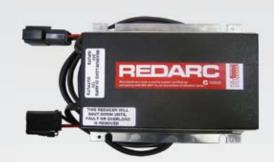
The 15-00508 Voltage Regulator operates in a 24 V DC automotive electrical system providing a safe 12 V output for 12 V equipment. It is a low noise voltage regulator designed for use with sensitive radio communications equipment. The maximum output is 20 Amps. The conversion efficiency at full load is more than 90%.
